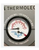
Once filling is complete, open the valve below the pump and unscrew all the blue connector valves. The injector will continue increasing the system pressure until it reaches between 12 psi and 15 psi.
