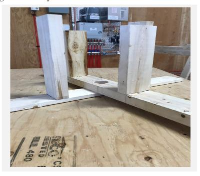
8~ Then, arrange the remaining one-by-four and two-by-four in the shape of a cross. Be sure the holes at the centre of the two boards line up. Set this piece aside.
