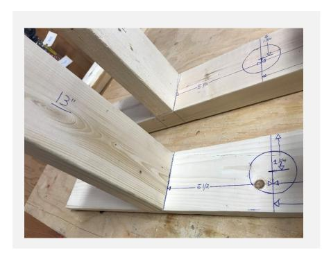
7~ Next, lay the one-by-four on the ground with the shorter two-by-fours sticking up. Lay the two-by-four on top, with the shorter two-by-fours sticking up. Align the holes at the centre of the two pieces and arrange them in the shape of a cross. Screw the one-by-four and the two-by-four together. This piece will serve as the hub of the uncoiler.
